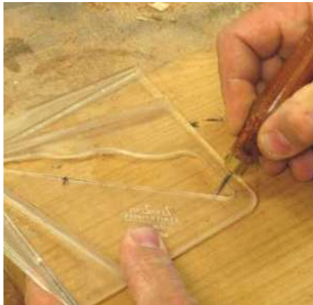
▲ Pic.2 Using a bradawl will allow you to get the best accuracy while marking the centre – this is better than a pencil. A cheap plastic centre finder is perfect for this job
